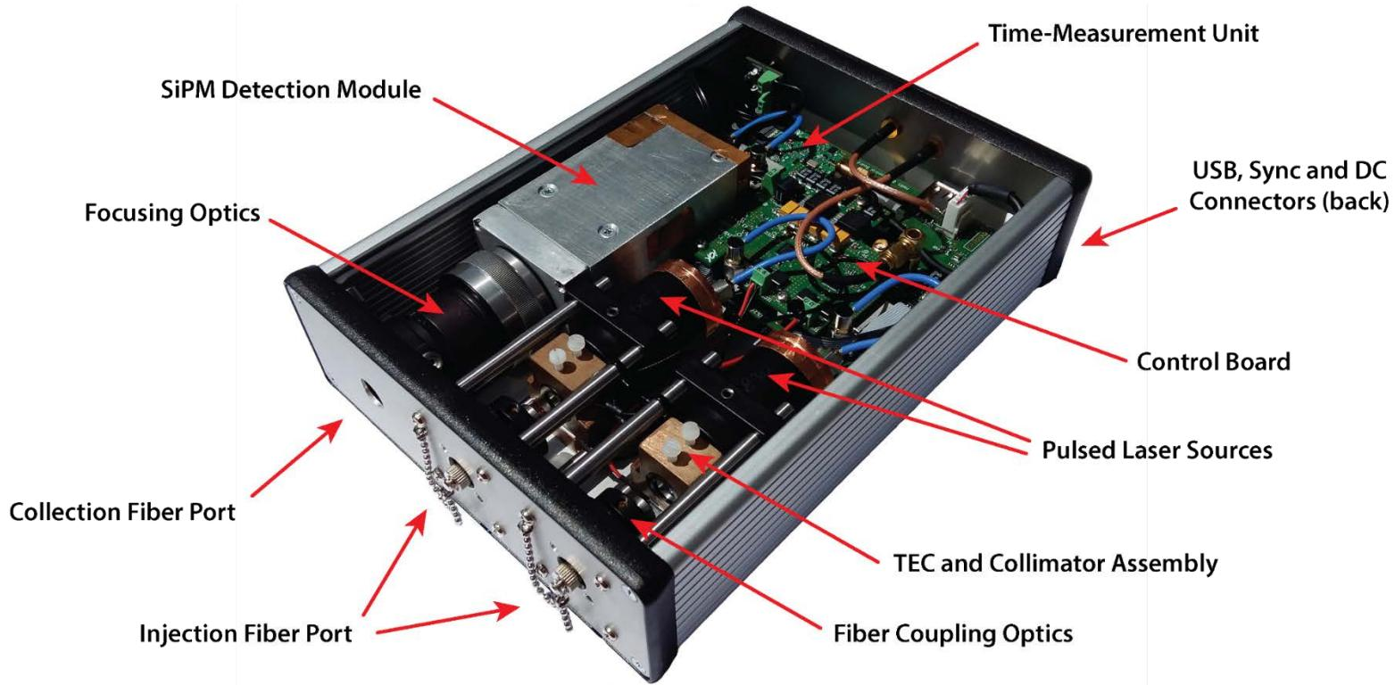
total power consumption lower than 10 W (ready for battery operation)
