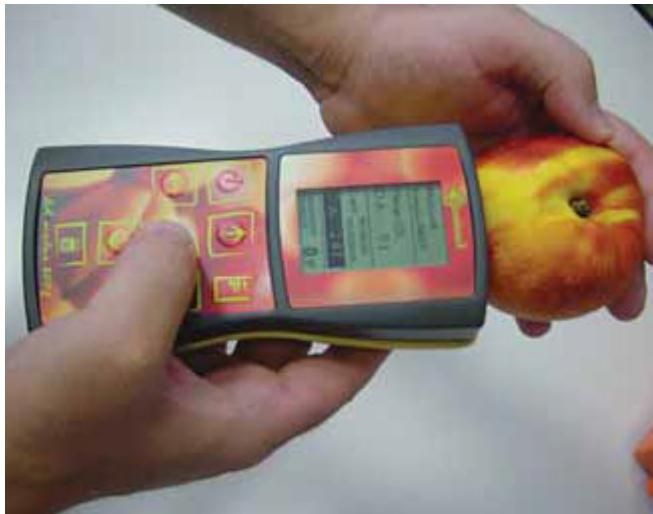
DA-meter, courtesy of P. Rozzi, Sinteleia (Italy)
